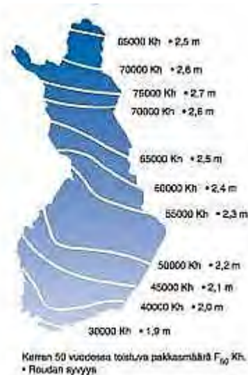
Figure 40: The dimensioning frost free depths for unheated buildings in Finland. Also dimensioning heating degree hours [Kh] are given. F_{50} gives the probability for these degree hours once in 50 years. [15]
